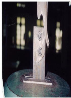
Fig 13 Block shear failure of single plain angle 40×25×3
