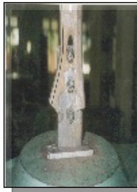
Fig 12 Tearing failure of lipped angle 60×25×15×3
