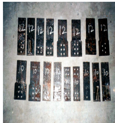
Figure 7 Gusset plates used for connection.
