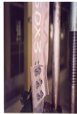
Fig 14 Net section fracture failure of plain angle 90×50×3
