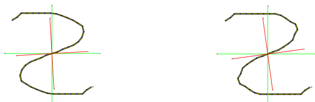
(a) P_n = 2.96 kips (b) P_n = 2.90 kips Figure 6 Optimal cross-sections found by SA for 16 ft column
