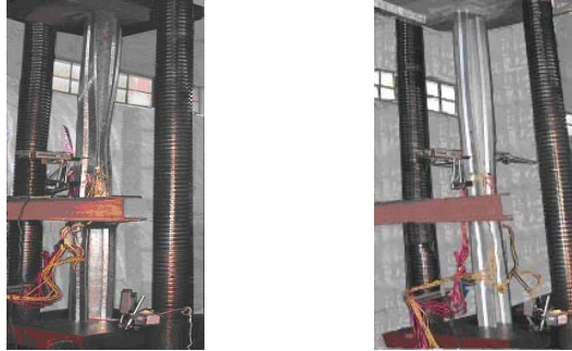
Fig.7 Buckling mode of longer specimens
