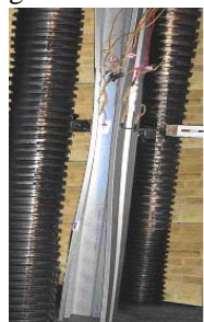
Fig.6 Buckling mode of medium-length specimens
