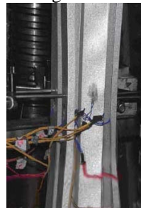
Fig.6 Buckling mode of medium-length specimens
