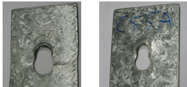
(a) Net section fracture, CS8b
