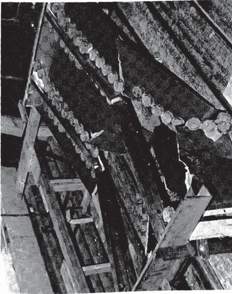
Fig. 25 Test G-1 After Failure
