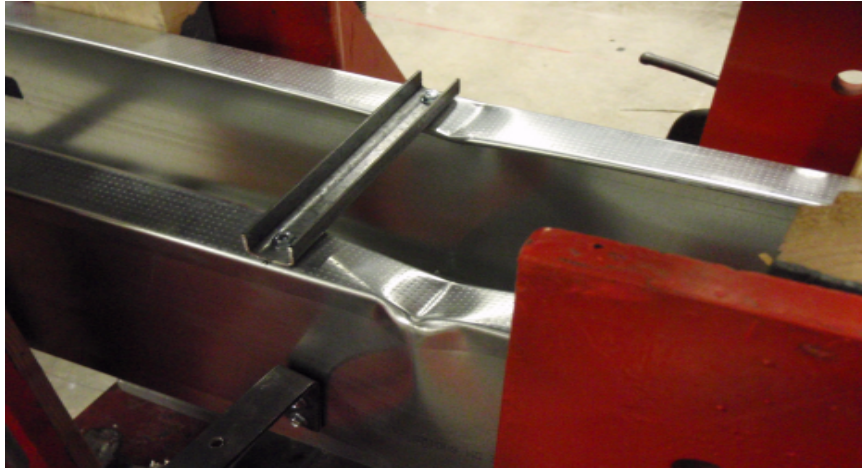
Figure 7: Typical flange buckling failure shown on a 6 in. (152 mm) specimen.
