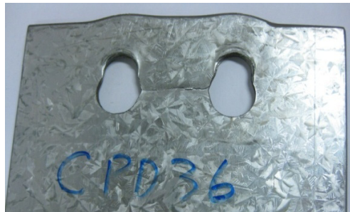
Figure 4 Shear-out deformations gave way to block shear failure
