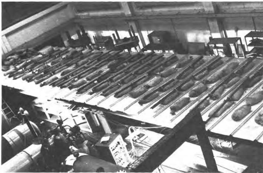
FIG. 5. TOP VIEW OF TEST ROOF (LIVE LOAD TEST)
