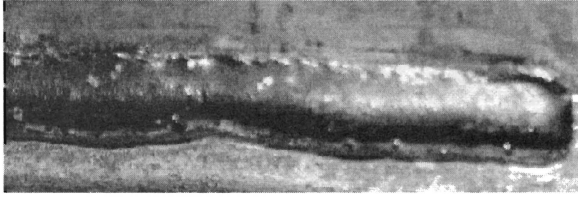
Fig. 11 HAZ failure of a single-lap transverse fillet welded connection in 0.12-in sheet steel
