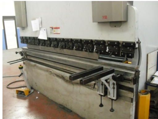
Figure 3. Press brake used to manufacture column specimens
