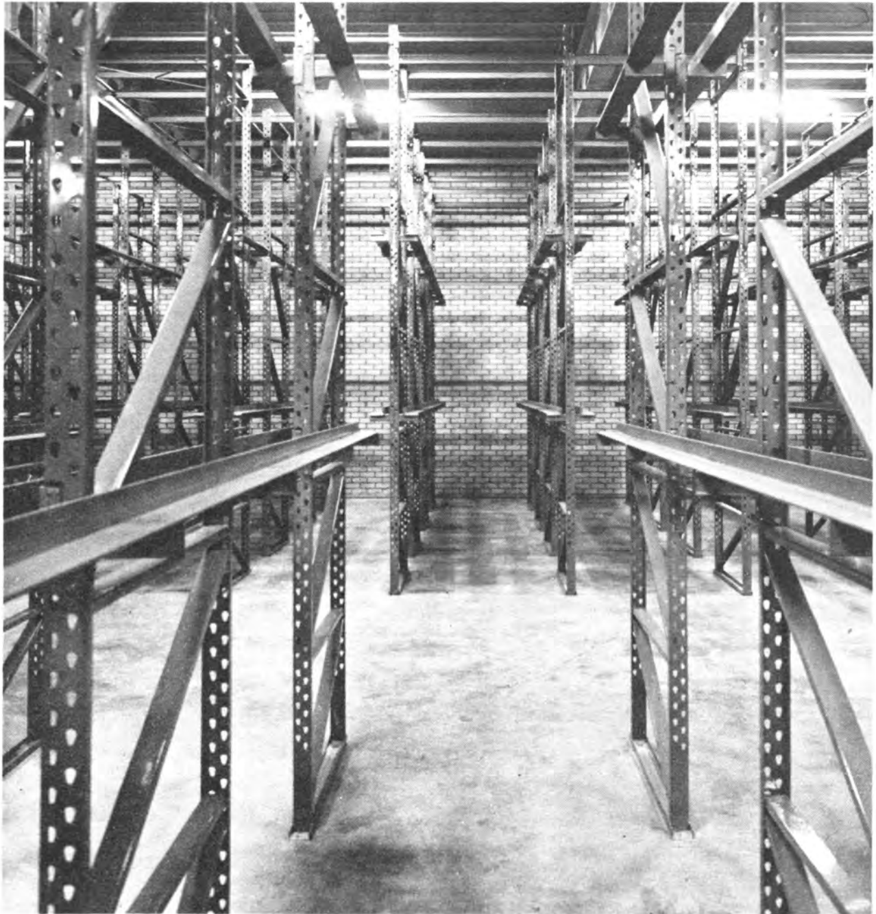
Fig. 2 Example of a drive-in and drive-through rack
