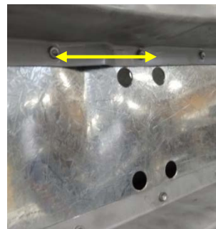
Figure 8: Web Buckling towards the Outside of the Beam, between Two Rivets, as found in 201x62x19x1.1x1.9 RHFCB with 100 mm Rivet Spacing
