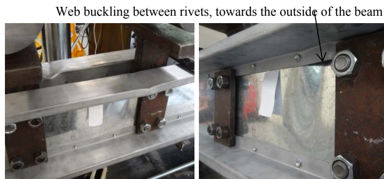
Figure 11: Failure Mode of 201x62x19x1.1x1.9 RHFCB with 50 mm Rivet Spacing
