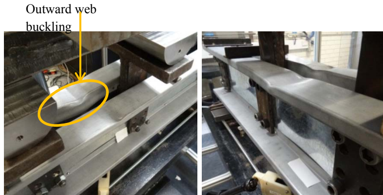
Figure 13: Failure Mode of 201x62x19x1.1x1.9 RHFCB with 200 mm Rivet Spacing
