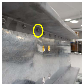
Figure 9: Web Buckling towards the Inside of the Beam, at Rivet Location, as found in 250x62x19x1.1x1.9 RHFCB with 50 mm Rivet Spacing
