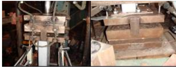
(a)Top support seat (b) below support seat Fig.6 The actual bidirectional-hinged support
