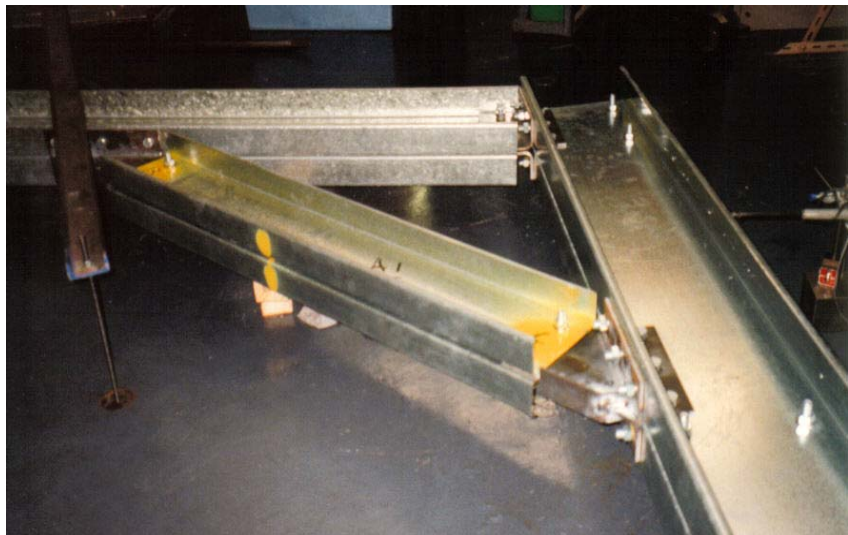
Figure 11 View of stanchion-rafter brace
