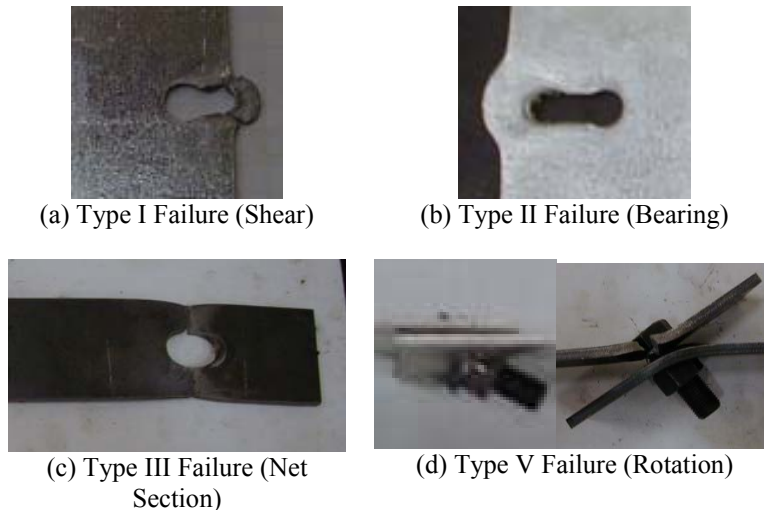
Figure 3 Photographs of Observed Failure Modes
