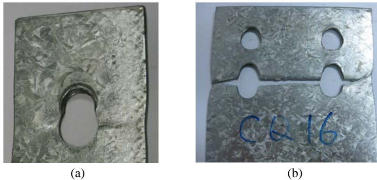
Figure 1 Net section tensile ruptures in flat sheets
