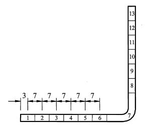
Figure 2: Positions of tensile and residual strain coupons
