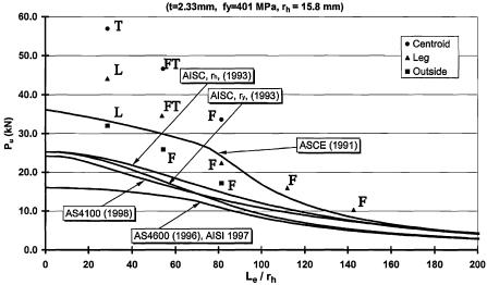
L50x50x2.5 Compression Parallel with Leg - Pinned Ends (t=2.33mm, fy=401 MPa, r<sub>h</sub> = 15.8 mm)
