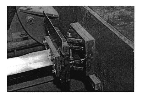
Figure 6: Pin-ended bearing
