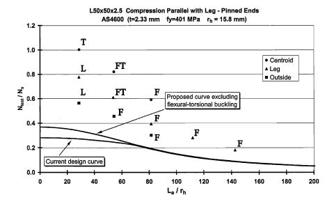
Figure 8: Test strengths vs AS/NZS 4600 and AISI design curves,  $(N_s=56.7 \text{ kN}).$
