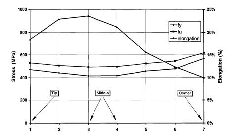
Figure 4: Stress and elongation distribution along leg width
