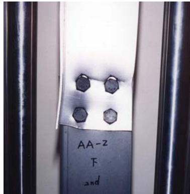
Figure 3 Typical Failure of a Specimen
