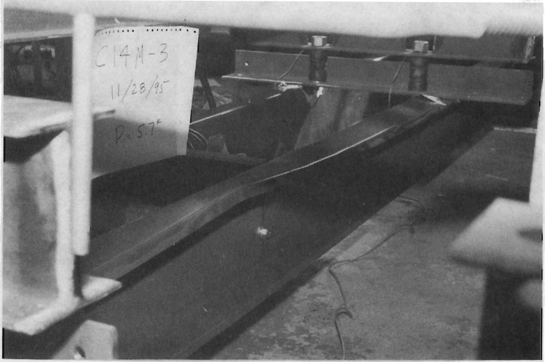
Figure 3(a) Distortional Buckling of Channel (Test C14M-3)
