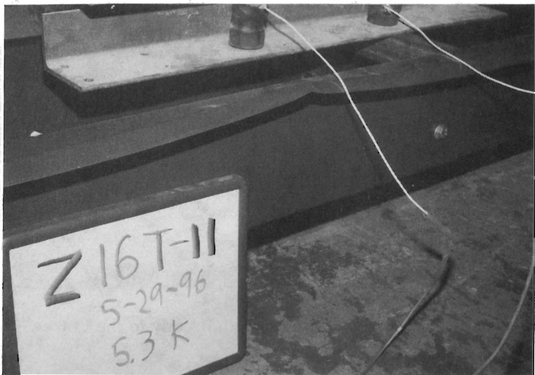
Figure 3(b) Distortional Buckling of Zee (Test Z16T-11)
