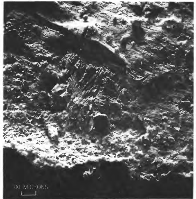
FIGURE 14.—Scanning electron microscope photograph of sand-bearing lignitic peat sample from core RTR2, 16.76 to 16.99 m. Note the isolation of sand grains in an organic matrix of plant fragments.
