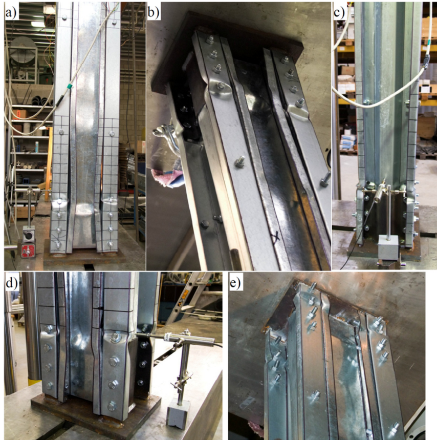
Figure 7. 2x\Sigma200+2xC145 failure mechanisms: a) distortion of C-section and plastic deformation at bottom base; b) top base; c) distortion in \Sigma -shape; d) deformation at bottom base; e) deformation in welded specimen.
