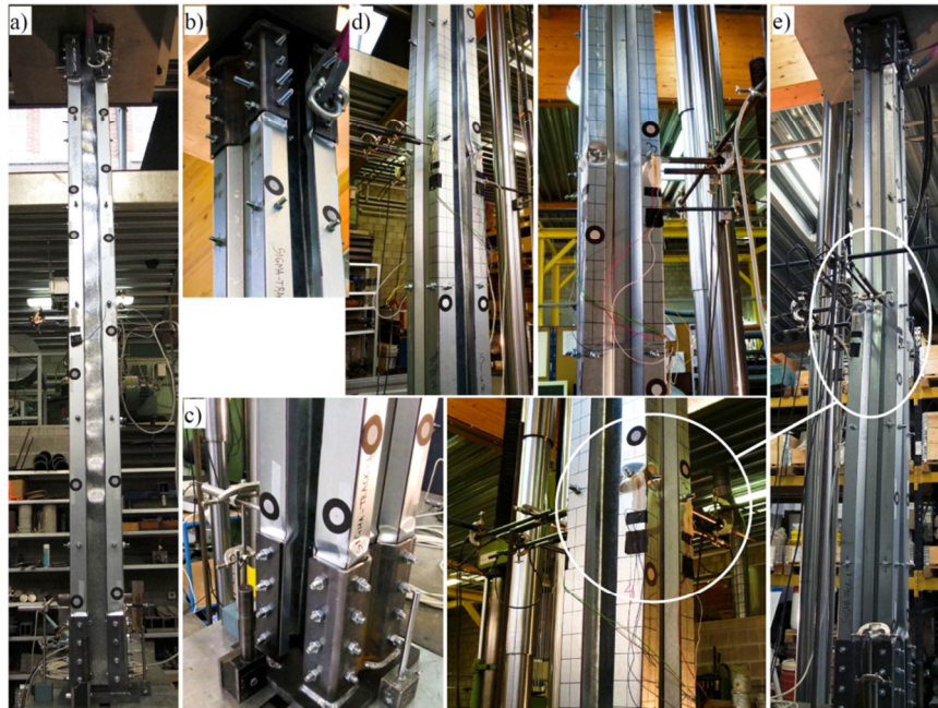
Figure 5. 2xΣ200+2xTr195 – failure mechanisms: a) overall deformation and plastic local buckling in the track profiles; b) and c) plastic deformation at connection pieces; d) distortion and yielding at mid-height; e) overall deformation due to distortion at mid-height.
