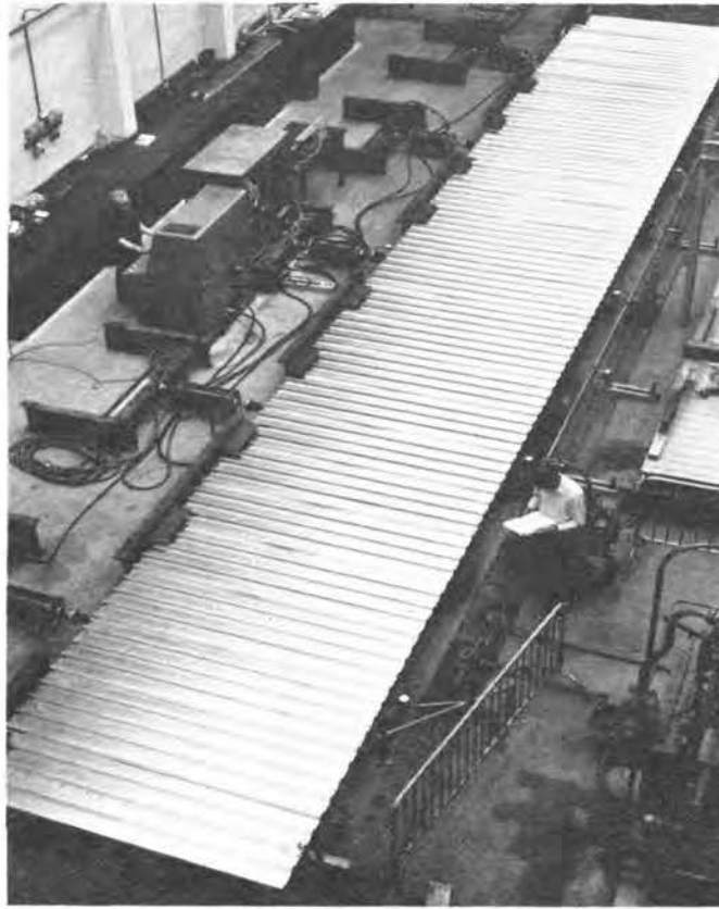
Fig 13 Stressed skin girder under test.
