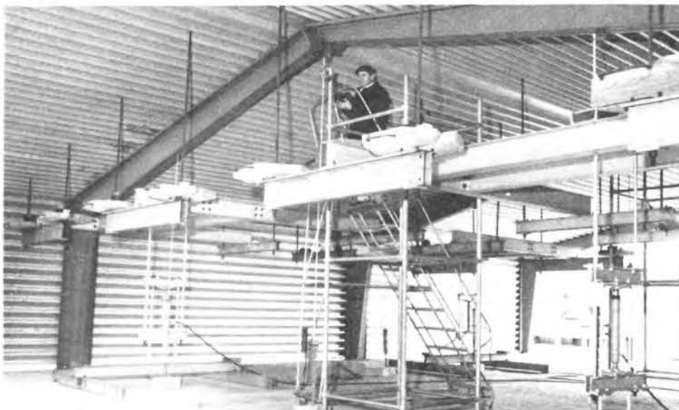
Fig 7 Interior of test structure showing loading system.
