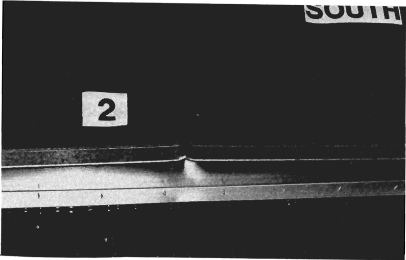
FIG.4 FLANGE-WEB LOCAL BUCKLE
