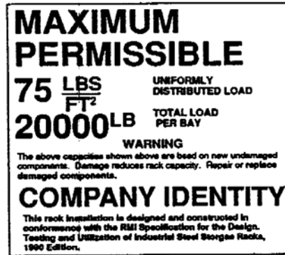
Figure 1.4.2b Example of Load Capacity and Compliance Plaque.
