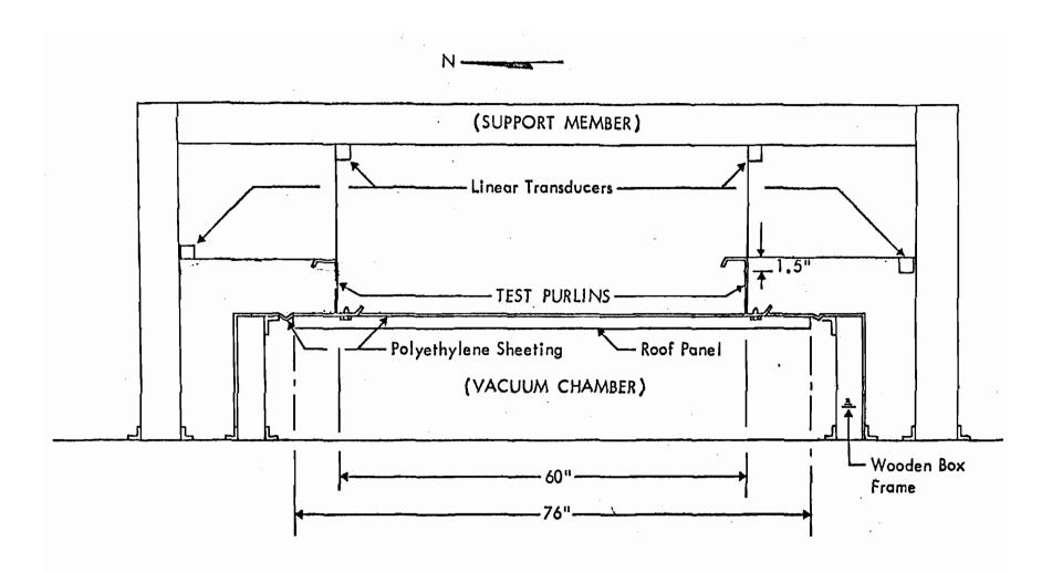
Figure 2 - Cross Section of Purlin Uplift Vacuum Test Chamber
