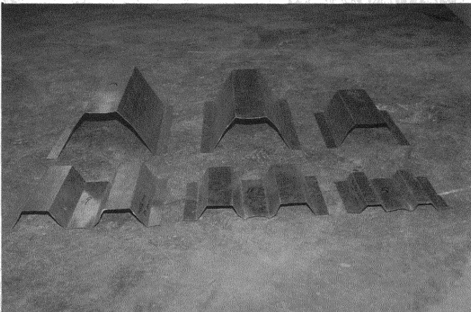
Fig. 4.5.2 Failure of Specimens after Tests in ETF Condition
