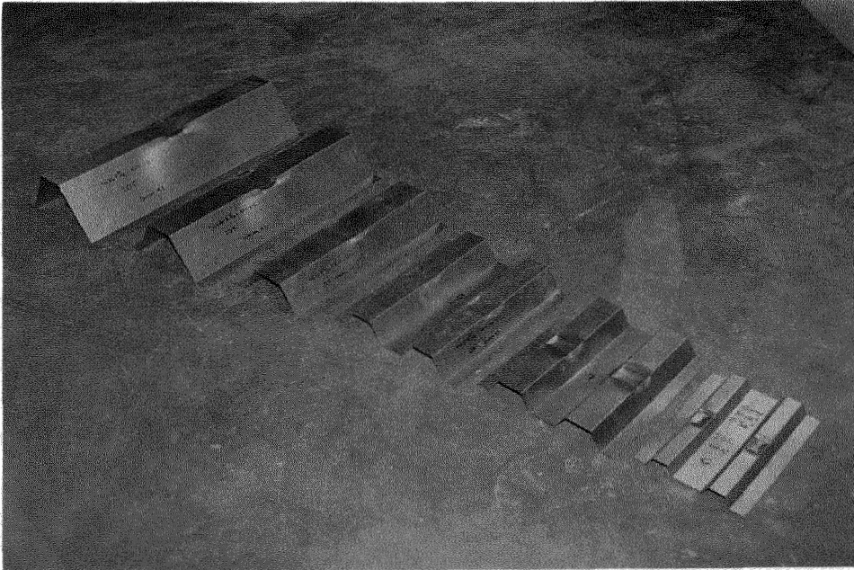
Fig. 4.4.6 Failure of Specimens after Tests in IOF Condition
