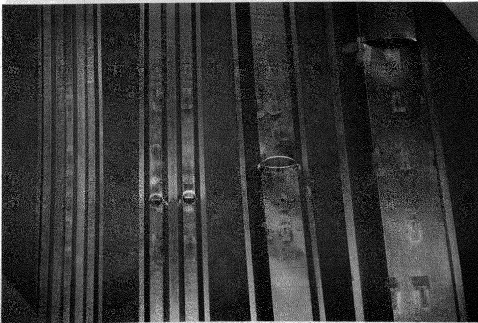
Fig. 4.4.8 Failure Mode of Panels in Two-Point Loading Condition (Continued)
