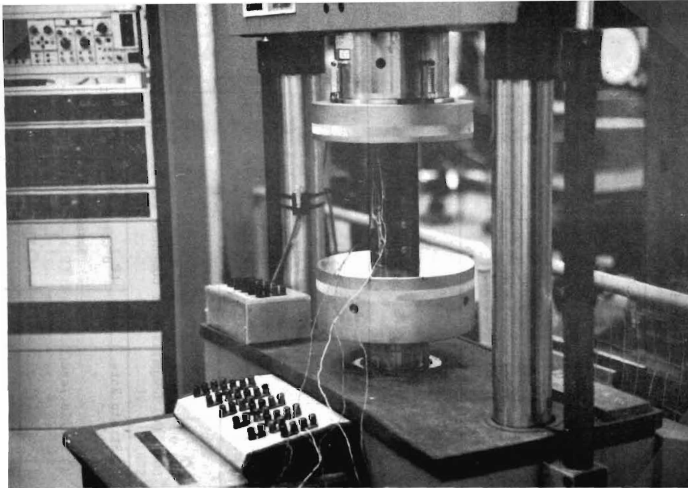
Figure 4.47 Photograph of an I-Shaped Stub Column Specimen Assembled by Bolts (Spec. 2B3AA)
