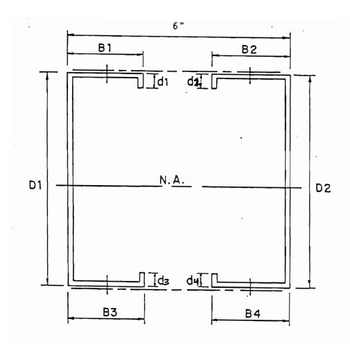
Figure 2. Beam Cross-Section
