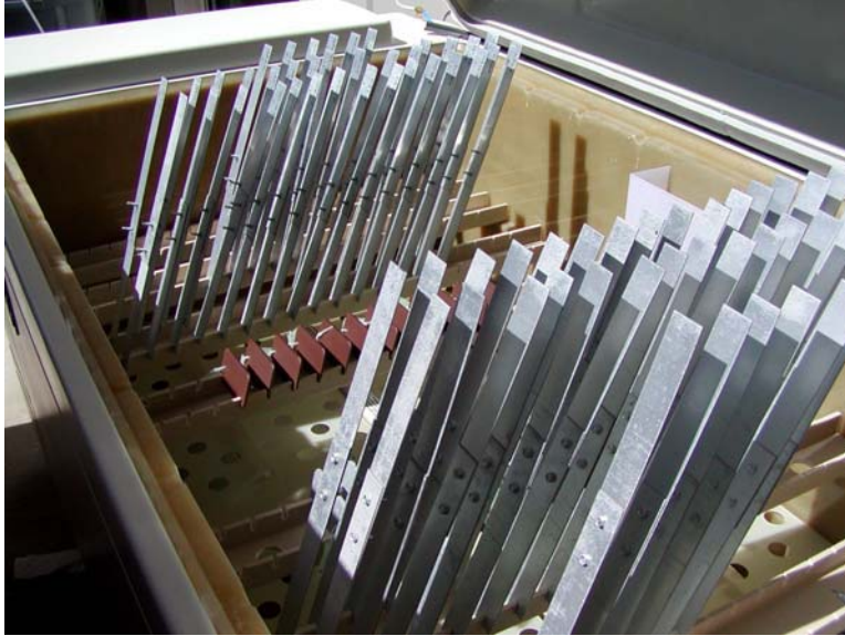
Figure 5.16: Test connections in the corrosion chamber
