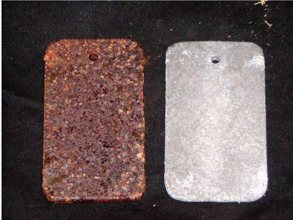
Figure 5.12: Steel and zinc coupons after 3186 cycles in the corrosion chamber.
