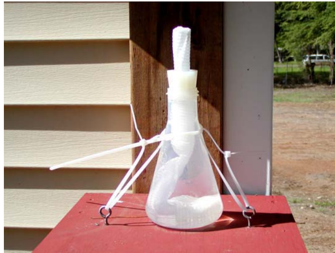
Figure 2.23: Atmospheric Chloride Candle.
