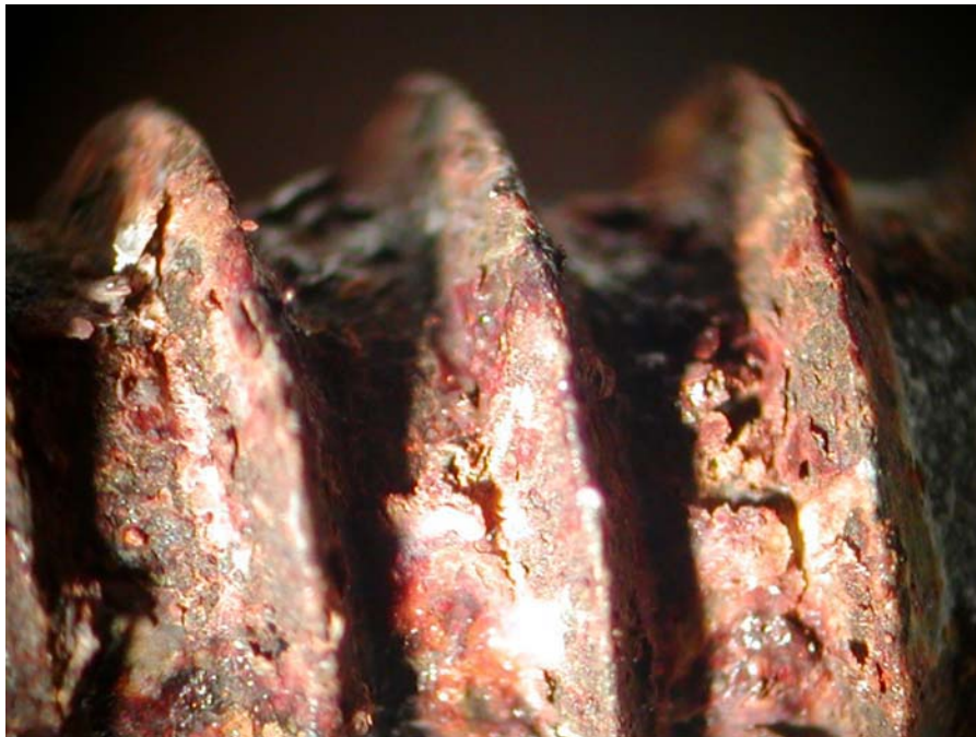
Figure 6.38: Screw threads after 1537 cycles in the corrosion chamber.
