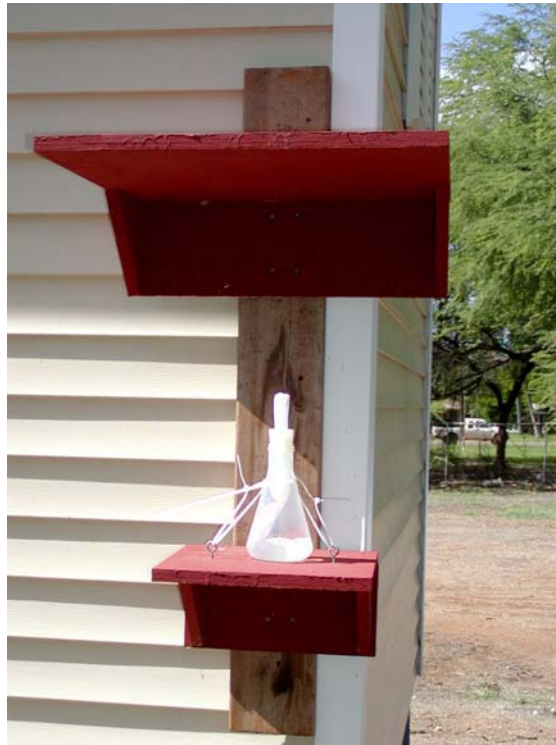
Figure 2.24: Atmospheric Chloride Candle and Shelter.
