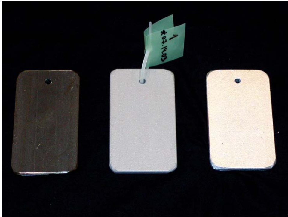
Figure 5.9: Steel, sand-blasted steel and zinc coated steel coupons (Left to right)
