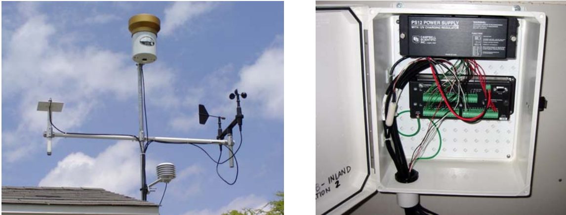
Figure 2.17: Weather station external sensors and datalogger
