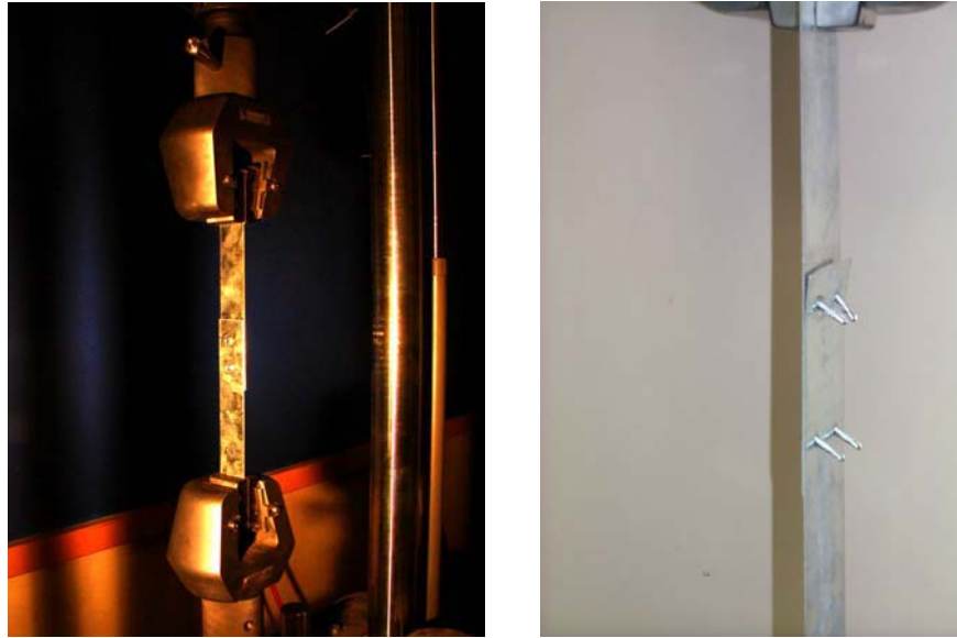
Figure 4.5: Test Specimen in Test Frame.
