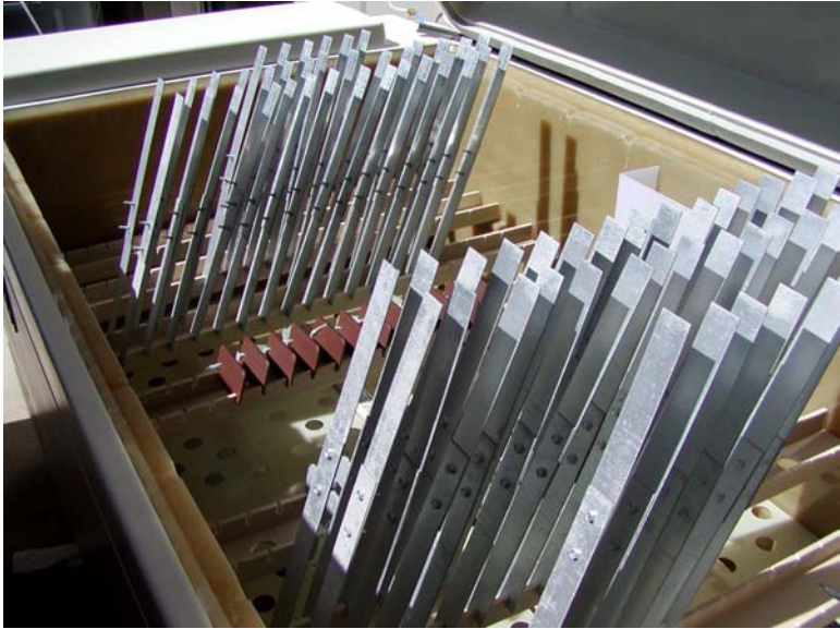
Figure 5.16: Test connections in the corrosion chamber
