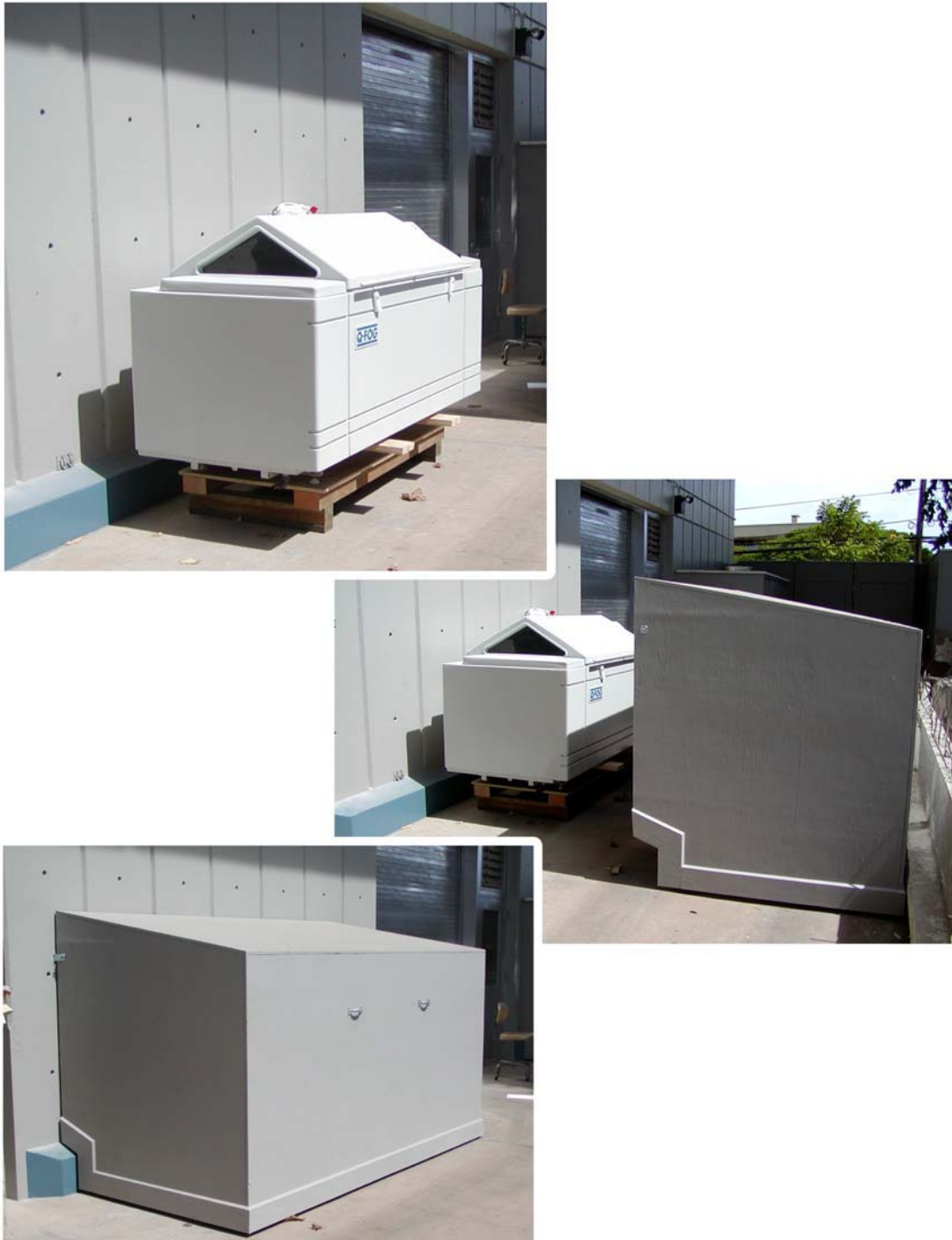
Figure 5.2: Corrosion chamber adjacent to Structures Lab
