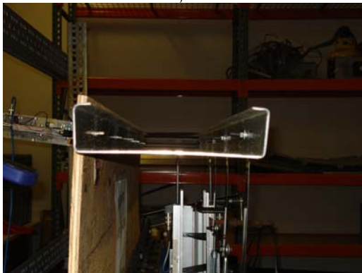
800S200-097 just prior to load
