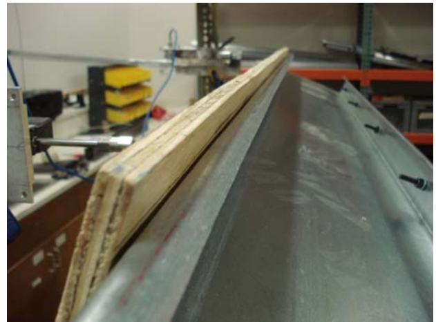
(d) separation between plywood sheathing and joist flange for 800S200-97 joist with plywood, L = 12 in., and #10 @ 12 in. fasteners (1-PL-12-10-12-03, 1-800S200_97_4B)
