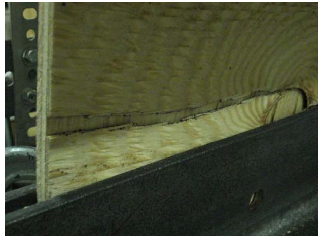
(b) failure in plywood initiating at a knot shown for 800S200-54 joist with plywood, L = 12 in., and #6 fasteners @ 12 in. (1-PL-12-6-12-03, 1-800S200_54_6(12))
