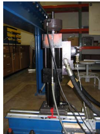
(b) hydraulic actuator on linear guide, load cell on top measures P , and internal LVDT measures \Delta_v
