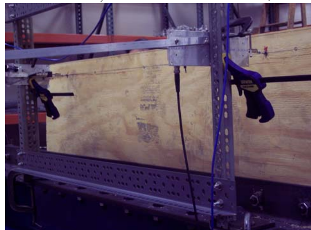
(d) rear view of L=12 in. plywood panel, position transducers mounted to frame and attached to back of panel for measurement of \Delta_{h1} and \Delta_{h2}
