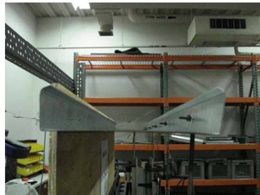
800S200-054 just prior to load
