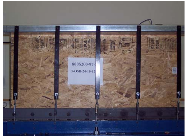
7/16 in. OSB in testing rig
