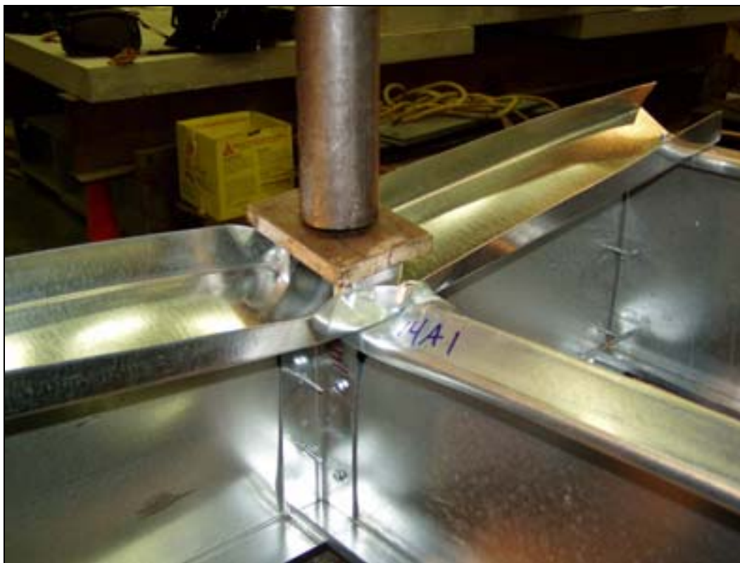
Figure 6.2 Tilting of Loadbearing Stud
