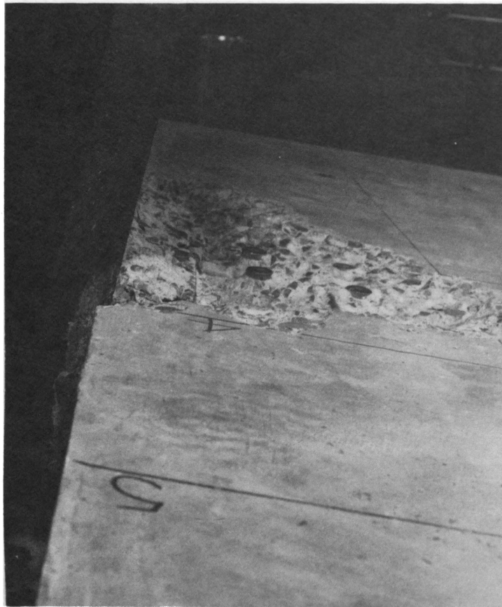
Fig. 39b B-64: Side View of Failure Surface
