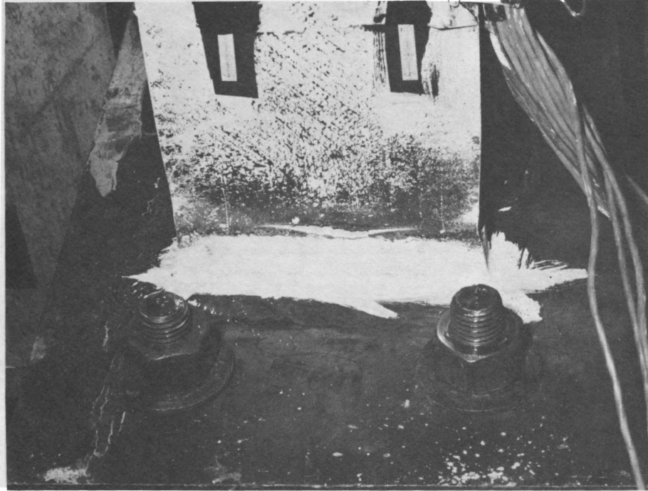
Fig. 59a Cracking of the Tension Flange of Test G1
