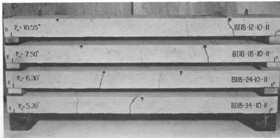
Fig. 6. Failed beam specimens for casting numbers 8, 9, and 10 using 18-gage steel form I.
