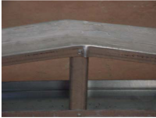
Figure 4.13 – Failure of Specimen 3D24-16
