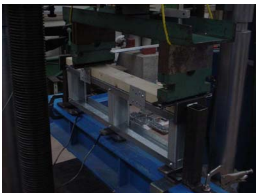
Figure 4.3 – Specimen 2A16-18 with shear plates
