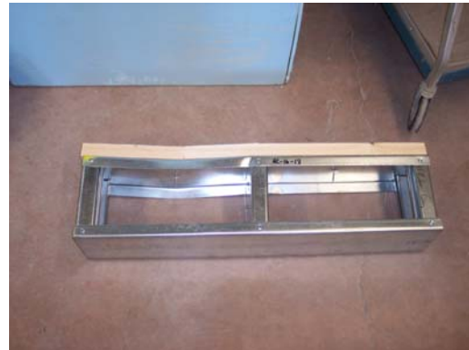
Figure 4.10 – Preferential Span Deflection, Specimen 2C24-18
