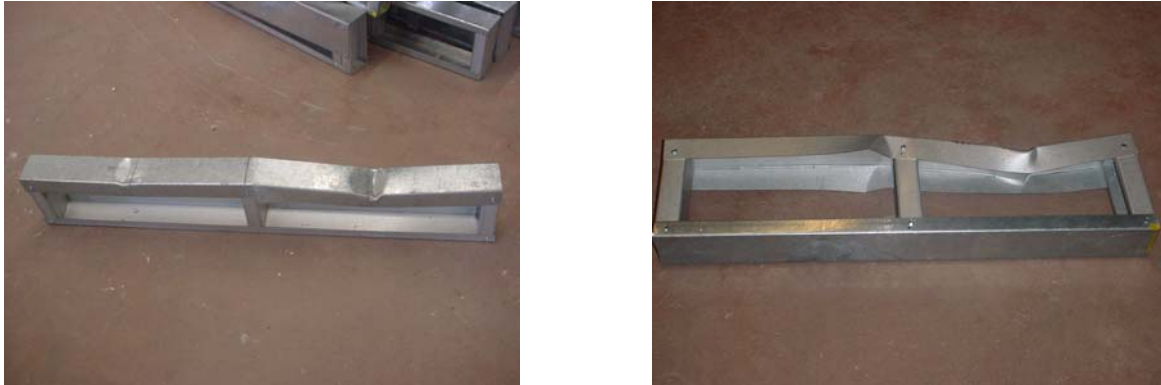
Figure 4.16 – Bearing Failures, Specimen Group E24-18
