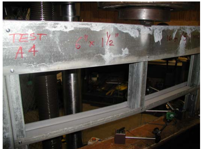
Figure 5 – Failure of Single L-Headers Tested Assemblies
