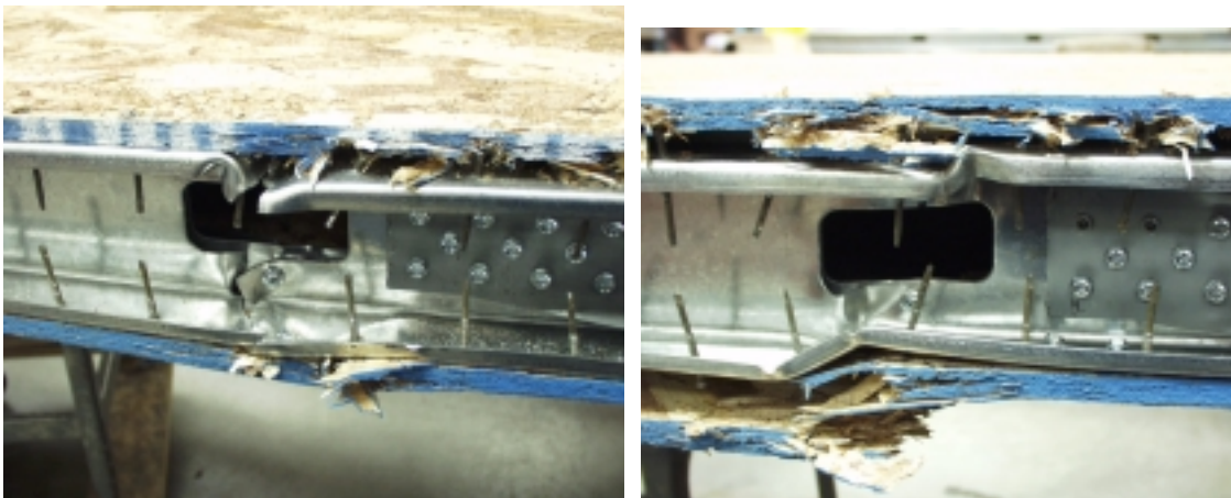
Figure 4. Observed behavior in Tests 6 and 7
