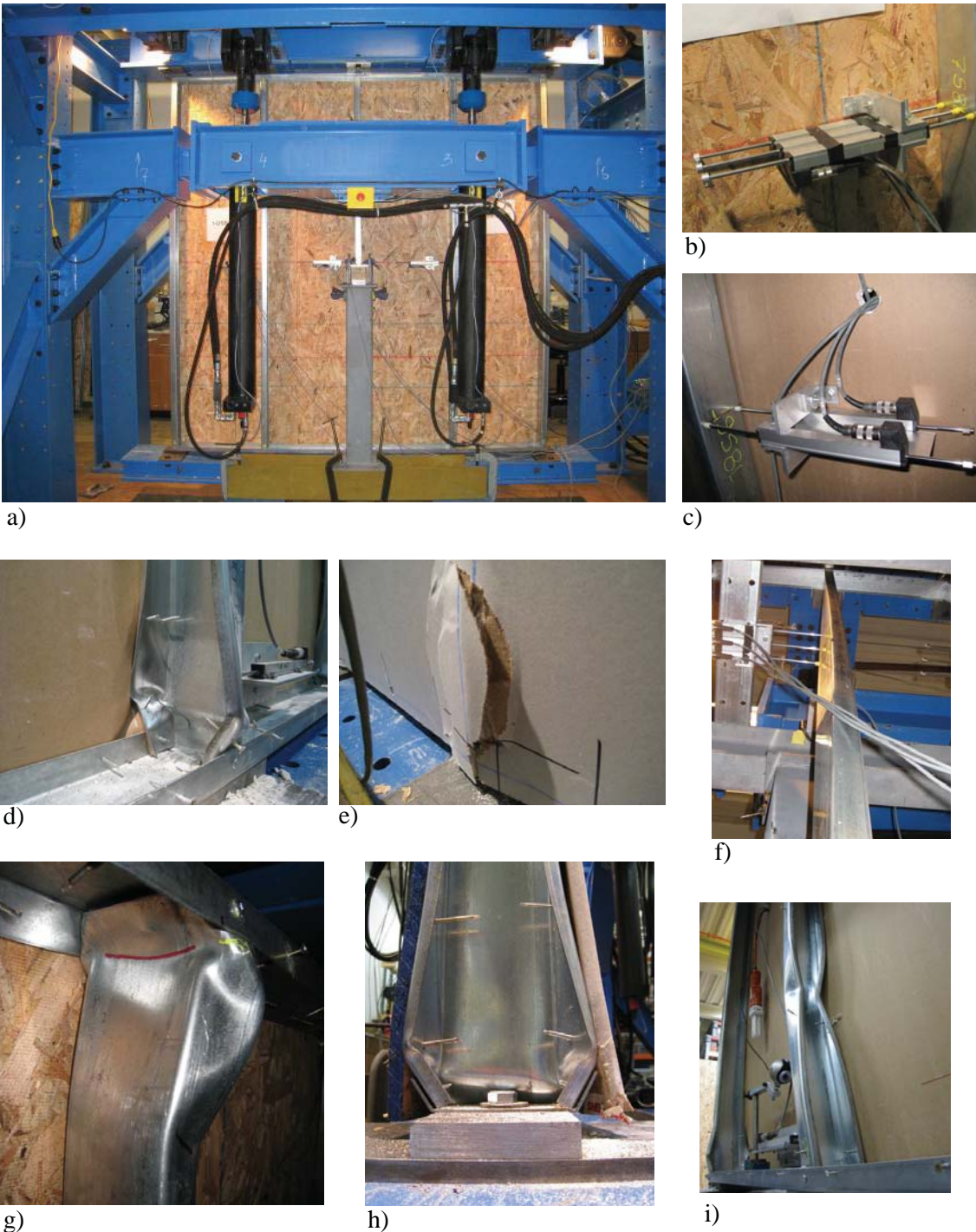
812 813 Figure 3 – Tests of sheathed cold-formed steel stud walls under compression: (a) side view of 814 wall in MDOF testing rig before testing; (b) and (c) PT sensors for measuring stud deformations; 815 (d) Gyp-Gyp wall opened after test to show local buckling at the ends; (e) local buckling tearing 816 gypsum board; (f) flexural-torsional buckling of unsheathed Bare-Bare wall; local buckling (g) at 817 the top of OSB-OSB wall, (h) at the bottom of OSB-Gyp wall, (i) followed by distortional 818 buckling on Gyp-Gyp wall.
