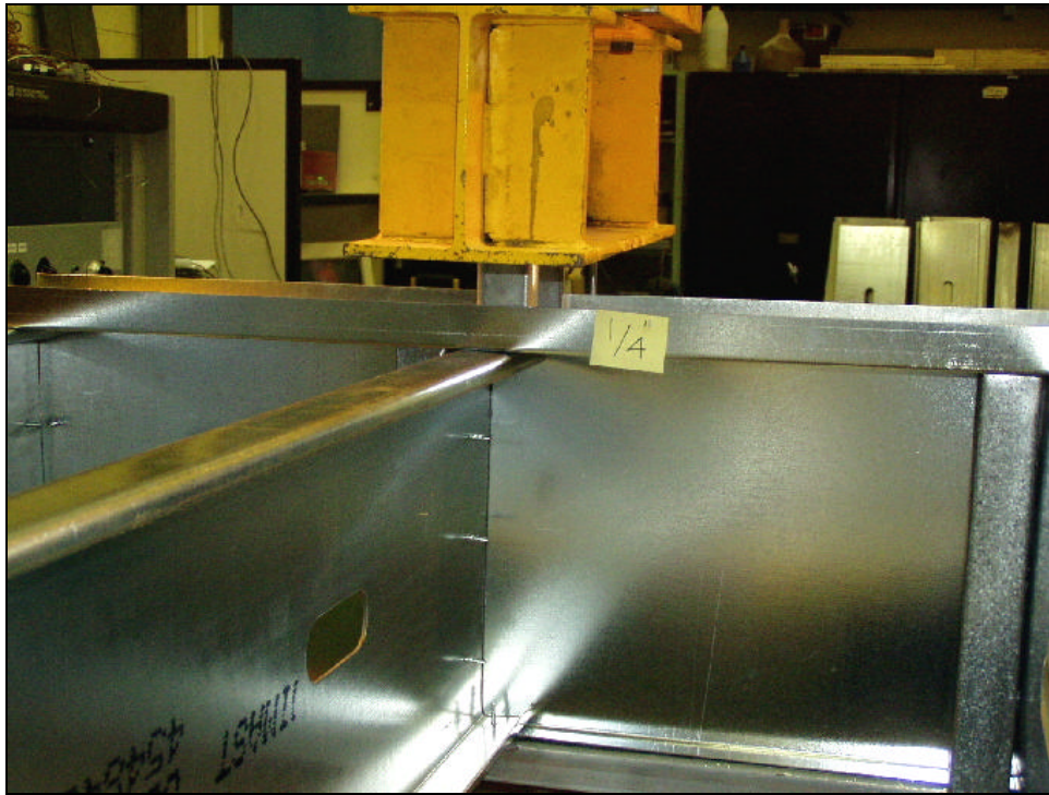
Figure 5.5: Photograph of the Deformation at \frac{1}{4} " Deflection (Offset Loading)
