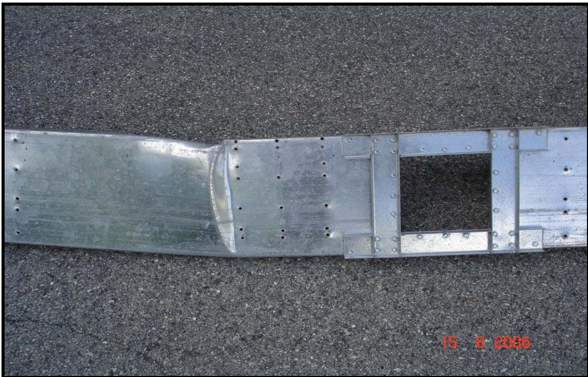
Figure C.3.6 Typical failure for specimens having reinforced (Scheme-“C”) square web openings
