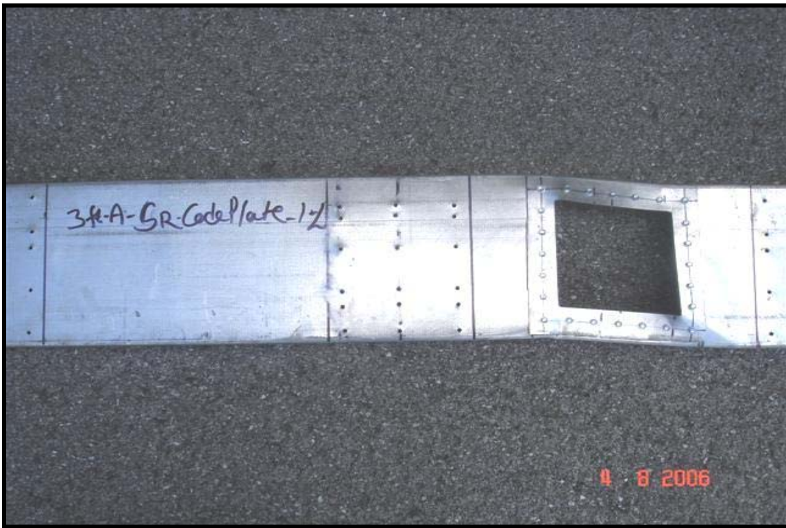
Figure C.3.2 Typical failure for specimens having reinforced (Scheme-“A”) square web openings
