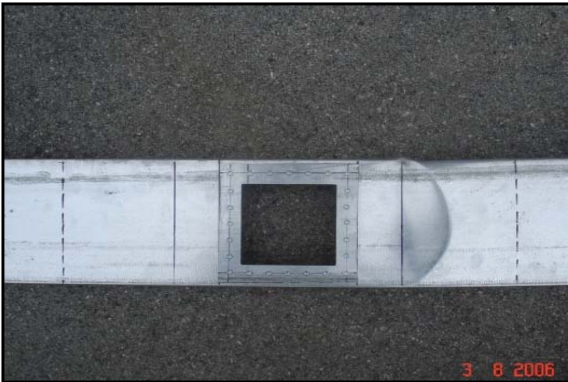
Figure B.3.2 Typical flexural failure for specimens having reinforced (Scheme-“A”) square web openings
