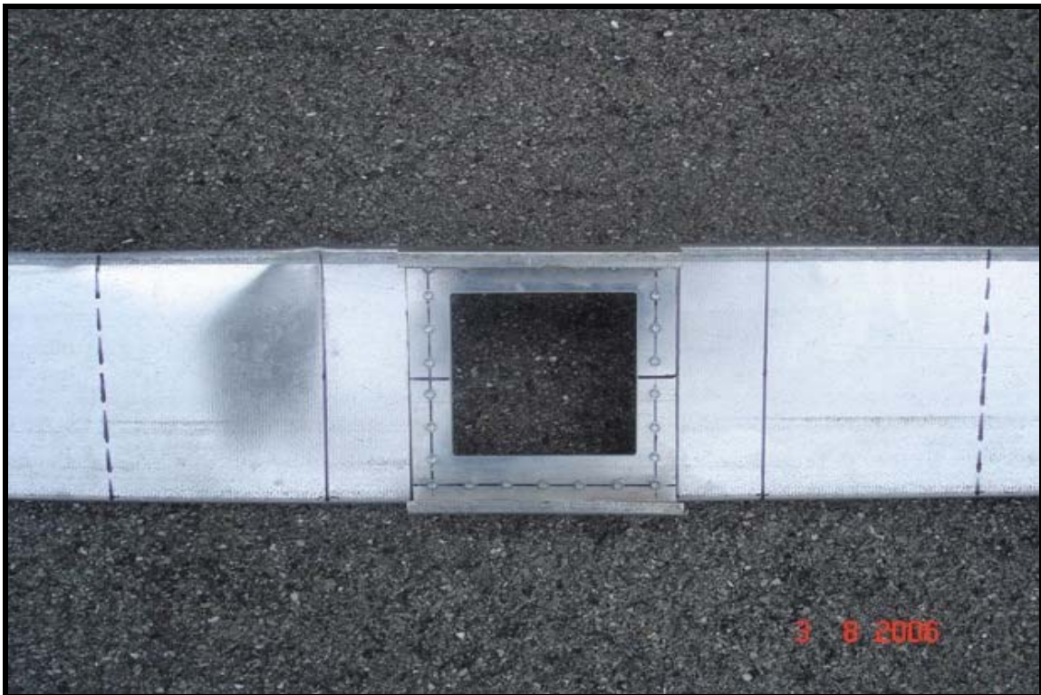
Figure B.3.4 Typical flexural failure for specimens having reinforced (Scheme-“B”) square web openings
