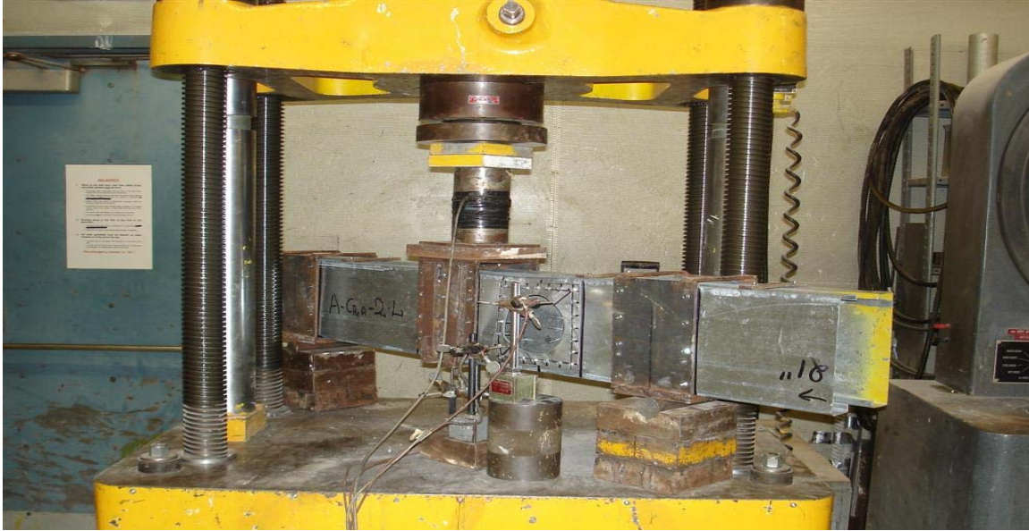
Figure 3.2 Photograph of the Shear Test Setup
