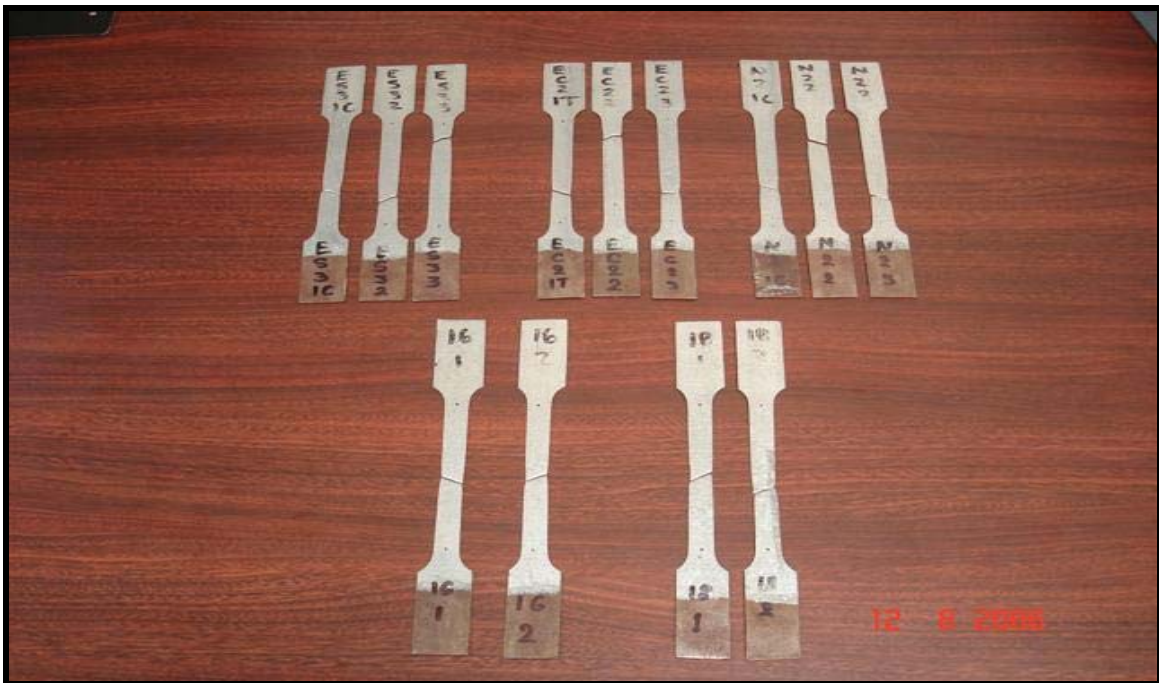
Figure A.4 Tension test specimens after testing
