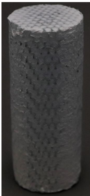
Figure 37: Final product with 3D structure and cellulose addition.
