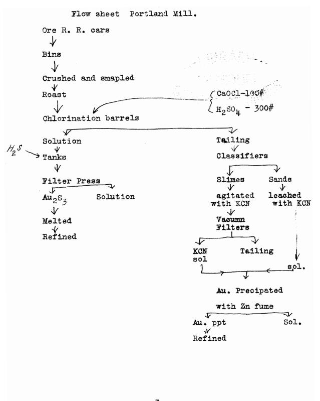
Many solutions of the problem presented by these low grade ores of Cripple Creek have been suggested and the failures are equal in number to the suggestions. The reason for failure seems due to the difference between the action of KCy., in gold and on the telluride of gold.
