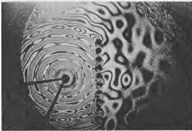
Fig. 35: Isolation effect of rows of bore holes, holographic interferometric (Woods, et al., 1974)
