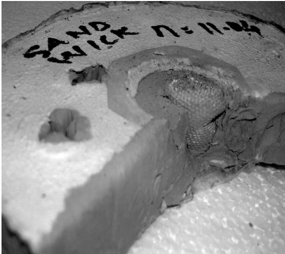
Fig 14. Kaolin clay sample with central sandwick at the end of consolidation
