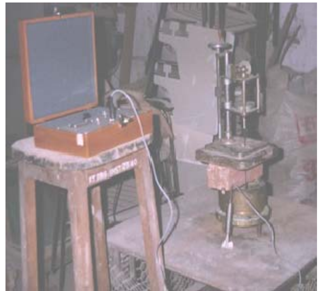
Fig.3. Shaking table with oedometer, vane shear and vibration meter
