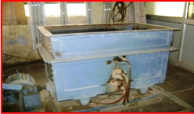
Fig. 1: Liquefaction Table at Dept. of Earthquake Eng. at IIT Roorkee
