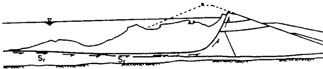
Fig. 17. Post-Liquefaction Deformed Shape of Lower San Fernando Dam (Seed et al., 1988)
