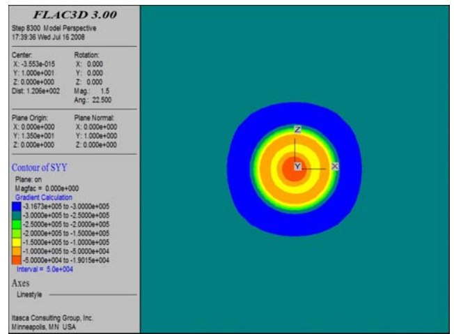
Fig. 13. Contours of vertical compressive stresses \sigma_{yy} below the rotunda, 13.5 meters below the ground surface.
