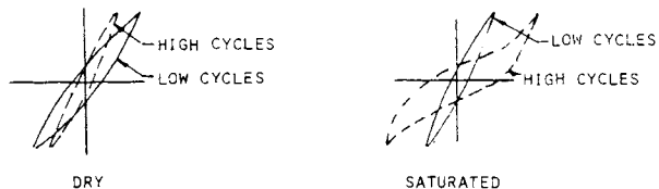
Fig. 1 Dynamic Non Linear, Hysteretic, Strain Dependent Soil Behavior.
