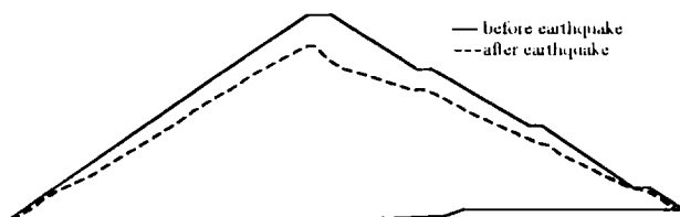
Fig. 15. Skeleton map of permanent deformation
